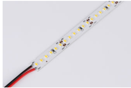
LT-2835W144Y-W24 Input:DC12V / 24V Power:16W/pcs LED:2835 144led/pcs Width:12mm Size:1000mm CCT:3000K/4000K/6000K RA:RA90
